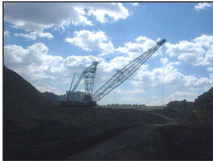
Figure 2.1: The Marion 1 dragline on location at the Syferfontein colliery.
