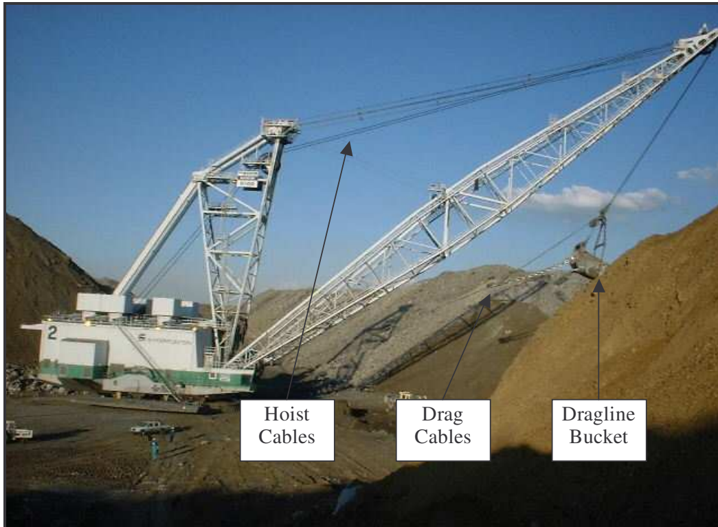
Figure 3.1: Layout of a dragline.
